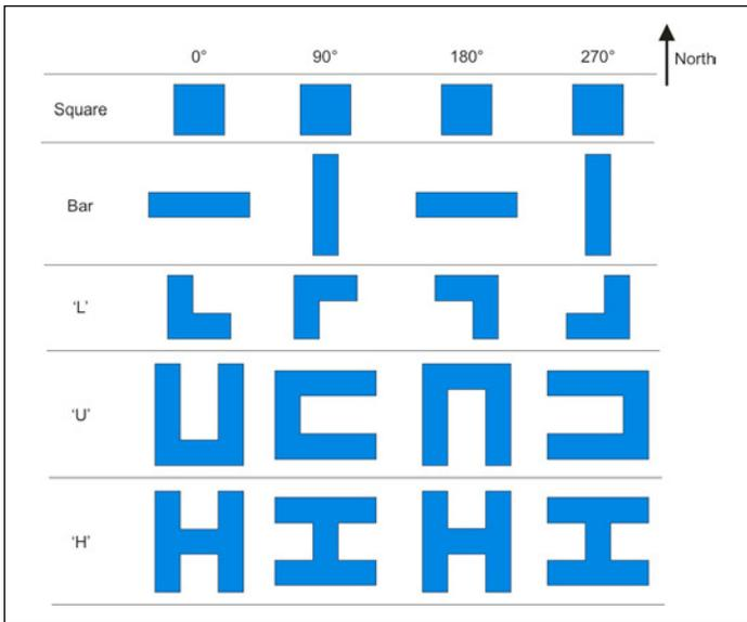
Figure 1 Building Floor Plates and Orientations Investigated
