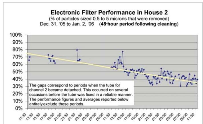
Figure 1 Degradation of filter performance in House 2
