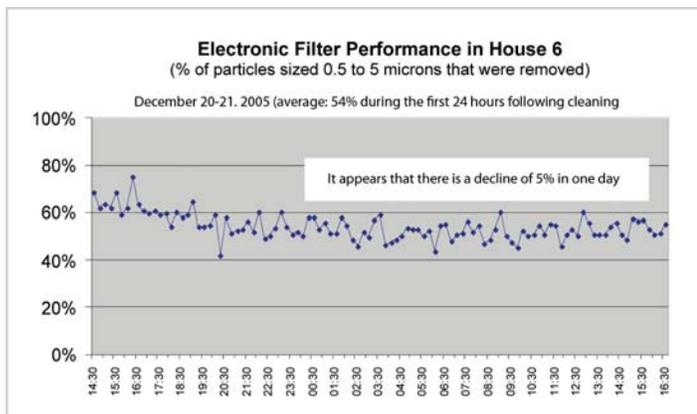
Figure 2 Degradation of filter performance in House 6
