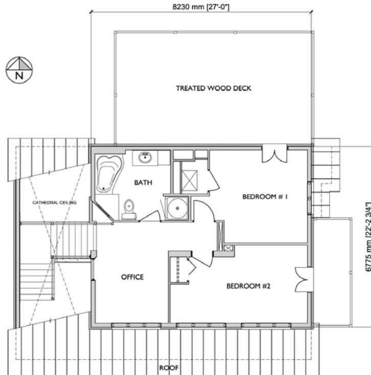
Figure 4—Second floor plan of ÉcoTerra™
