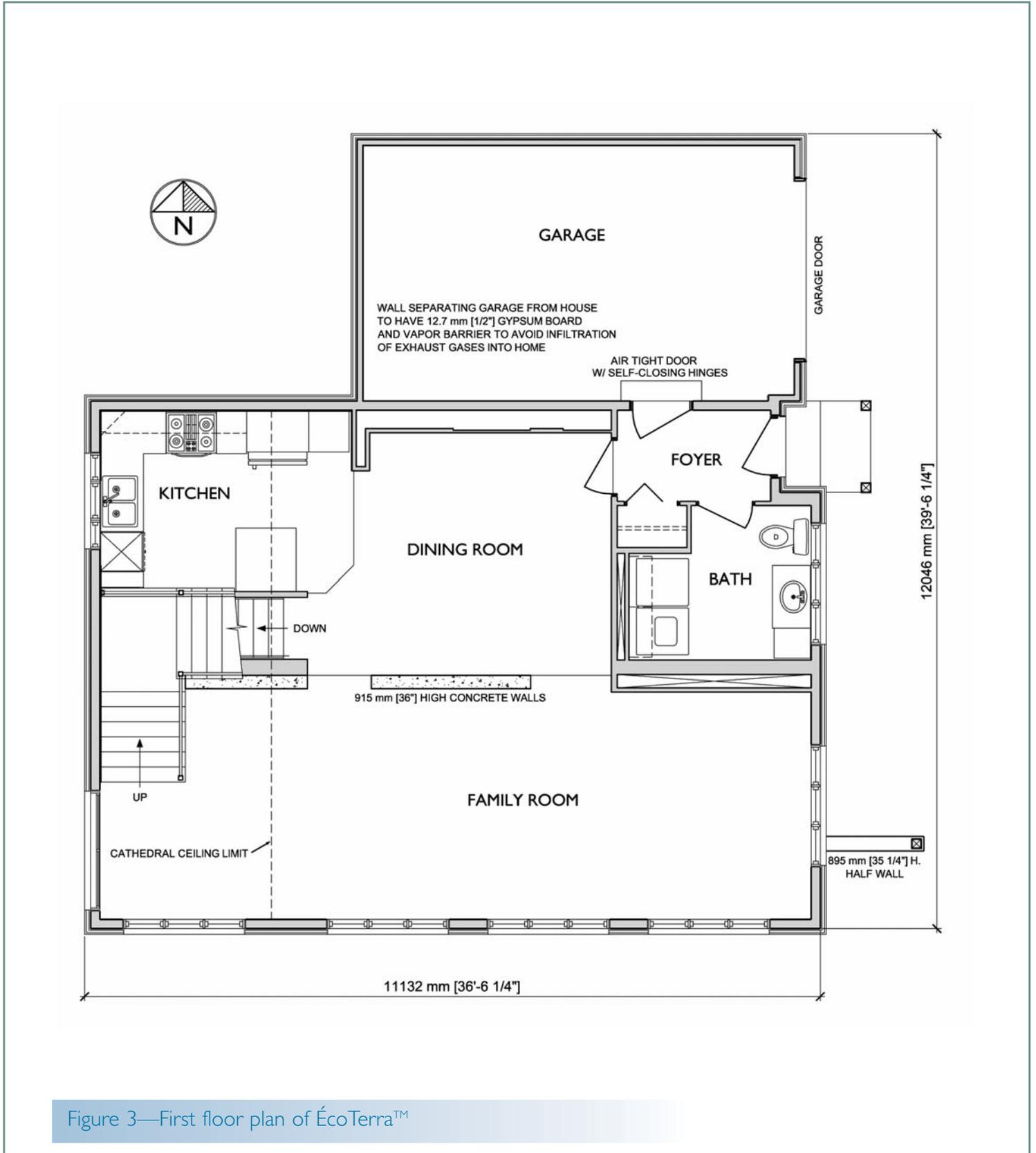
Figure 3—First floor plan of ÉcoTerra™
