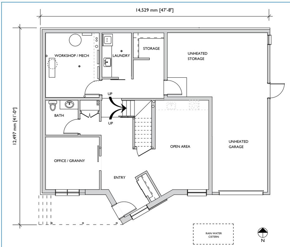
Figure 4—Lower floor plan of the EchoHaven EQUilibrium™ Project
