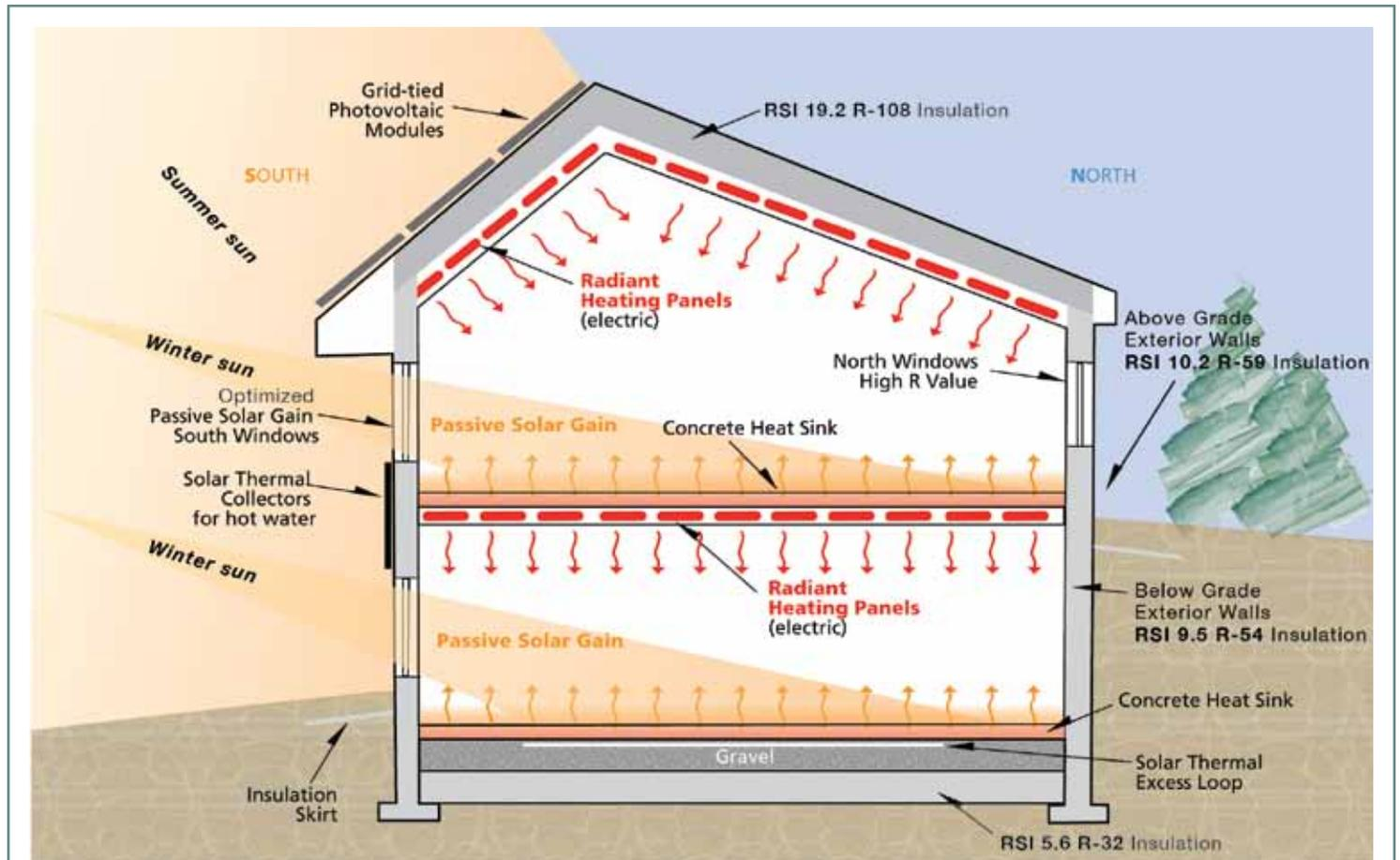
Figure 5—Cross-section of EchoHaven showing insulation and space heating sources
